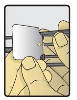
**Step 4:** Push down on the **trigger plate** to keep the **trigger wire** in place.
