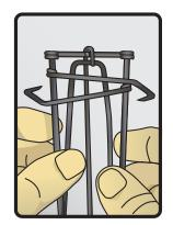
**Step 3:** While keeping your hand on the **trigger wire**, lift up the **trigger plate** to put the **trigger wire** through the **trigger plate**.
