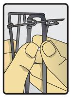
**Step 1:** Holding the trap in one hand, place the **trigger wire** through the bottom of the trap as shown.
