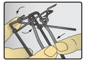
**Step 2:** Hold the **trigger wire** above the **trigger plate** with one hand. With your other hand, place your fingers underneath the trap and use your thumb to push the **loop** down to connect the catch around the **loop**. Keep applying pressure to the **trigger wire** to hold the **trigger wire** on the **loop**.
