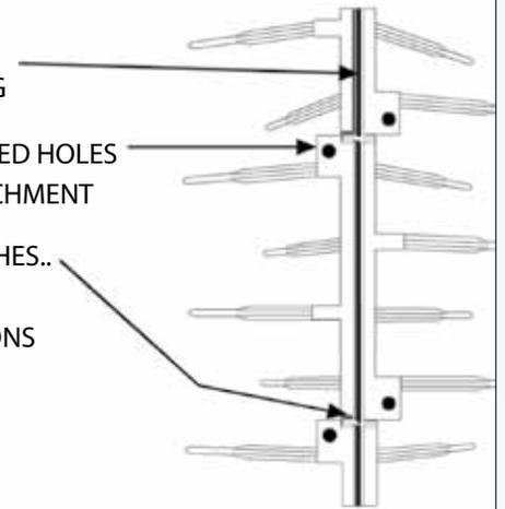
**To Install:** Surface should be clean and dry before installation. Select width of bird spike based on the surface to be covered leaving no more than 1" on either side for birds to land. Glue, screw or tie down to the surface.
