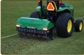
Step 1: Core aerify with multiple passes when conditions are proper to achieve maximum depth. Allow plugs to dry. Avoid aerification in high heat (80°+ F).
